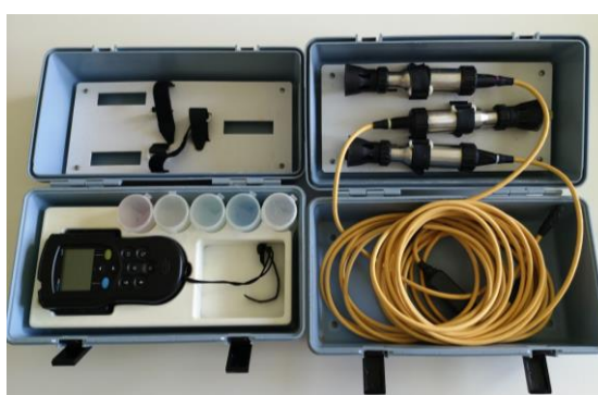
Figure 22: Hach HQ40D Portable Meter and three additional probes for measuring temperature, oxygen, pH, redox and electrical conductivity of the liquid
