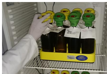
Figure 26: Measuring the BOD with a method that includes an electronic manometer (right)
