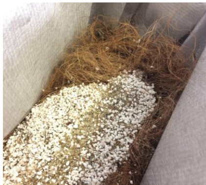
Figure 19: Materials used in the third bed: 2 mm geotextile fabric, 4 cm of substrate, 2 cm of coconut fibres covered with 14 cm of substrate. First, second and fourth bed had no layer of coconut fibres.
