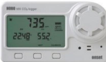
Slika 5: Merilnik HOBO MX CO2 Logger (MX1102) (Onset, 2017)
