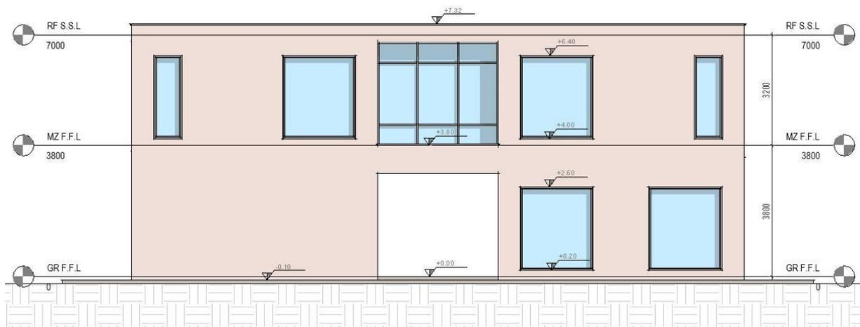
Figure 26: Back Elevation
