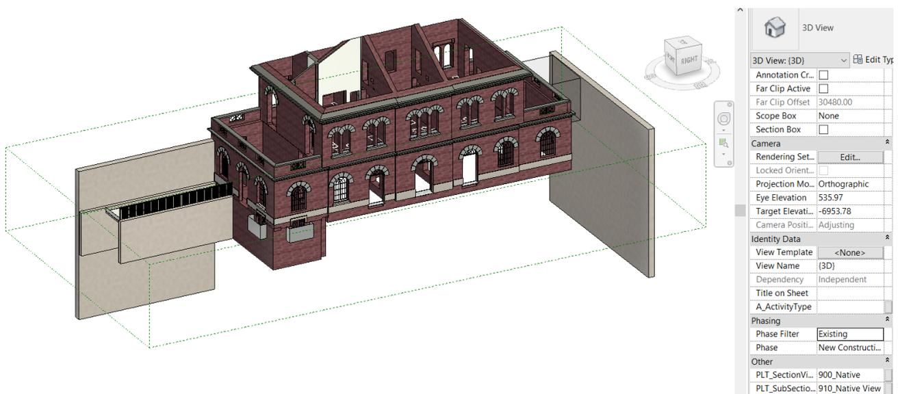
Figure 20 – Project Model filtered by Phase: Existing
