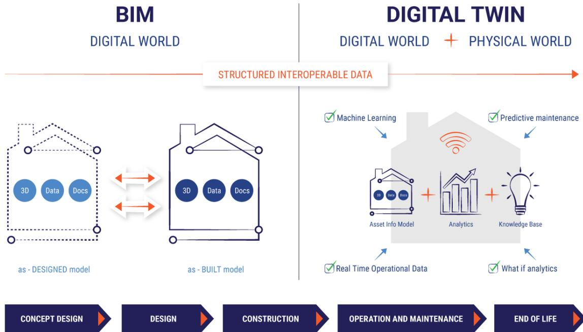
Figure 12 – Differences between BIM and DT (Cobuilder.com)
