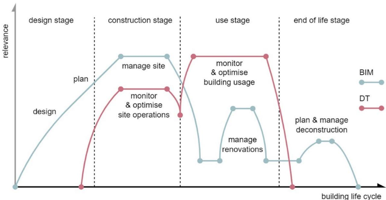
Figure 11 – Use of BIM and DT in the various phases of the project (Boje et al., 2023)
