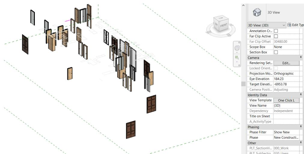
Figure 37 – Isolating elements through view templates
