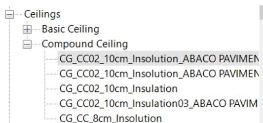
Figure 45 – Errors found in the naming of the ceiling's objects
