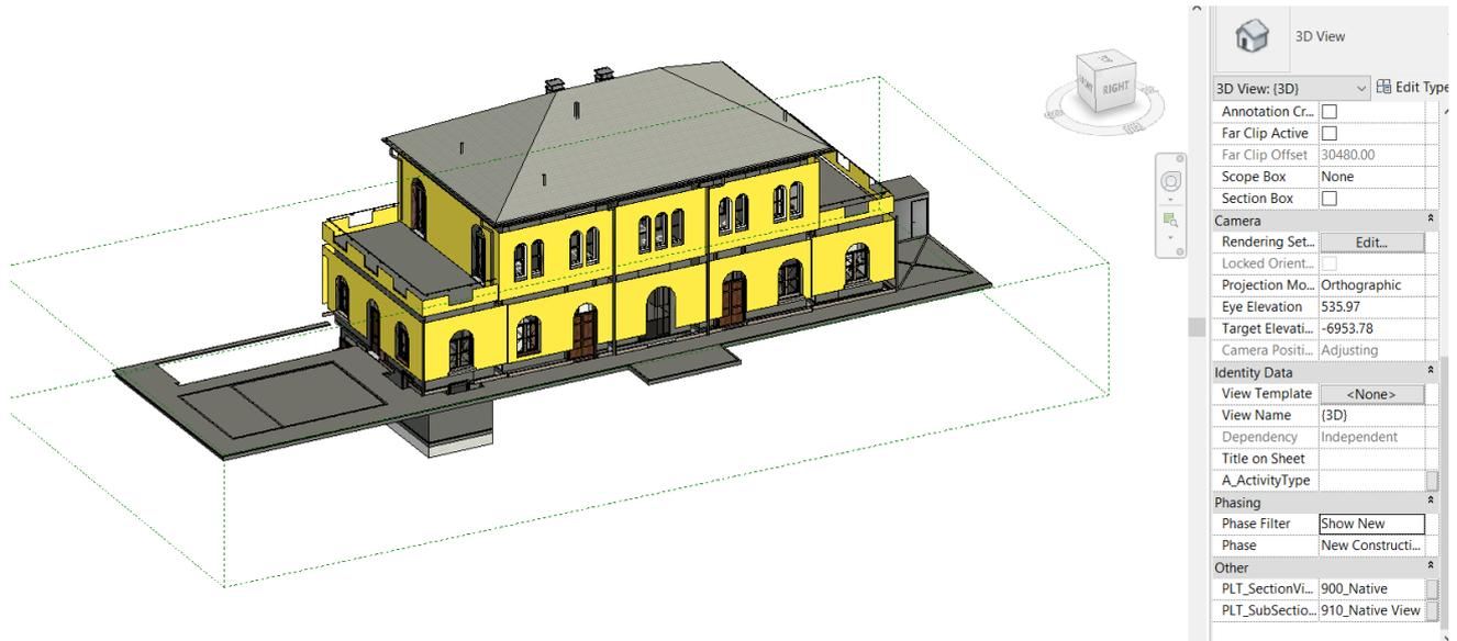
Figure 21 – Project Model filtered by Phase: New
