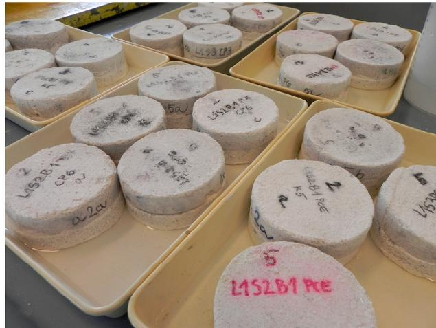
**Figure 5.** Sandwich discs exposed to capillary absorption of 3% NaCl solution.
