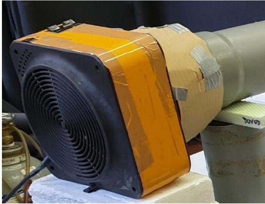
Figure 5.15: Electric heater.
