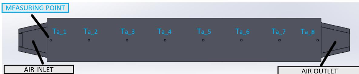
Figure 5.22: Locations of thermocouples for air temperature measurements.
