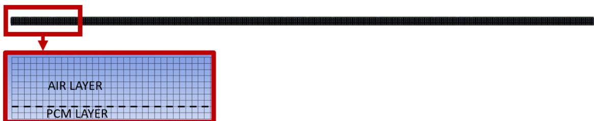
Figure 5.30: The selected grid with element size of 5 mm.
