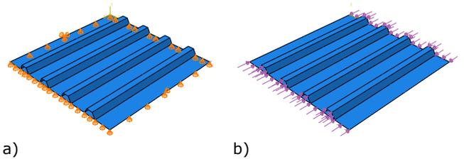
Figure 3 Numerical model for LBA: a) boundary conditions and b) loading [6, 11]
