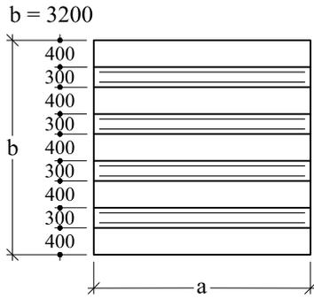
**Figure 4** Dimensions and arrangement of the stiffeners in panels of the parametric study [6, 11]
