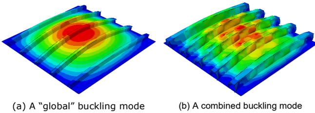
**Figure 1** Examples of buckling modes resulting from a linear buckling analysis (LBA) for a longitudinally stiffened plate loaded in compression
