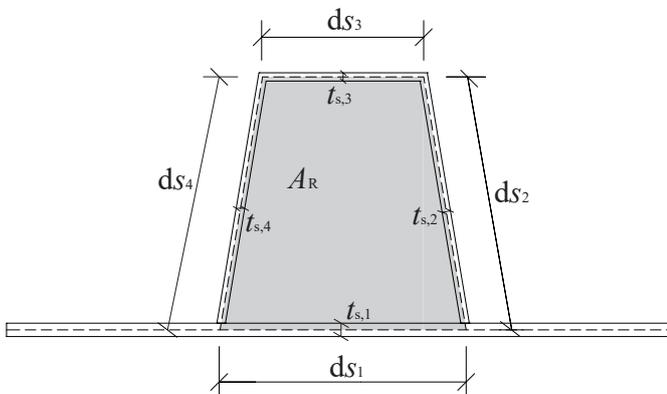
Figure 2 Cross-section properties of a trapezoidal stiffener
