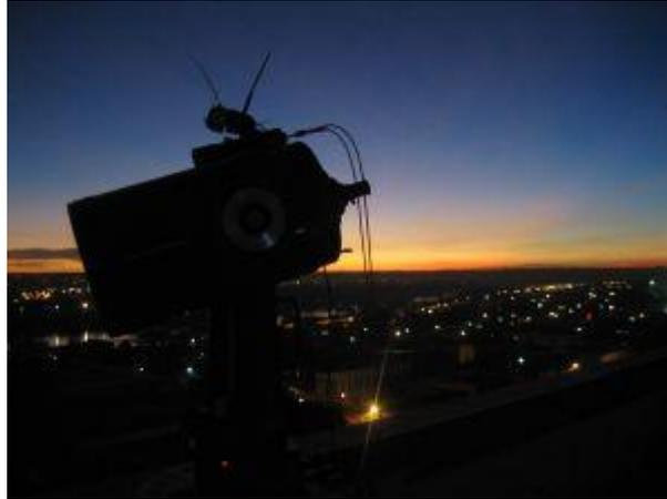
**Figure 3: Telescope of a ground-based spectrometer for the remote sensing of greenhouse gases. (KIT, 2011)**
