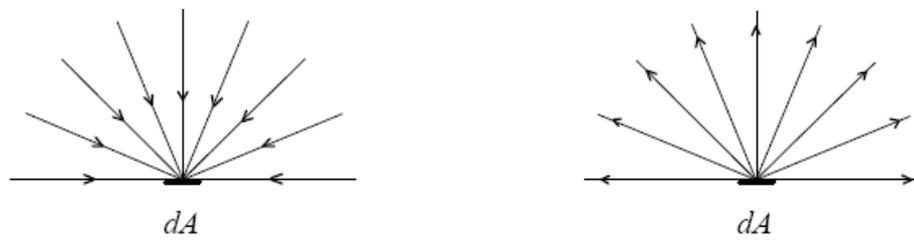
**Figure 13: Irradiance (left) is the electromagnetic radiation incident on the surface. Radiant emittance (right) is a term describing the radiation that is emerging from the surface. Irradiance and radiant emittance are radiometry terms for the power of electromagnetic radiation per unit area at a surface. The SI unit for both quantities are watts per square metre ( $\text{W}/\text{m}^2$ ).**
